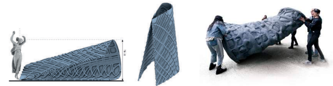
Left: Abstract Rendering of the enclosure with the 'rib-like' form. Right: Photograph of the form being repositioned into a standing orientation from the peeling one.
